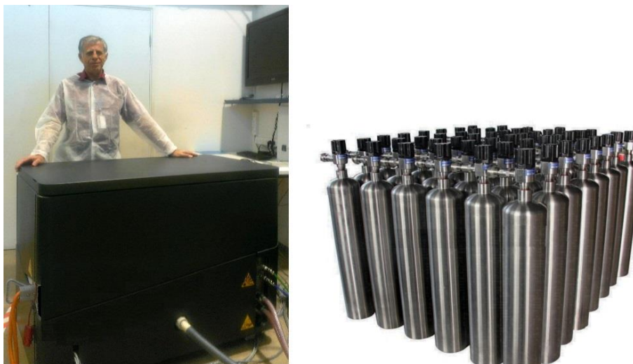
Fig. 5. 5 kW fuel cell and hydrogen storage metal hydride containers
